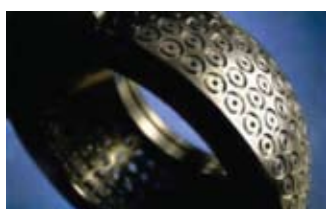
The Gamma Knife "helmet" is designed with openings that help focus the 201 radioactive sources.
